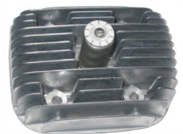
Cylinder head with ignition timing tool
